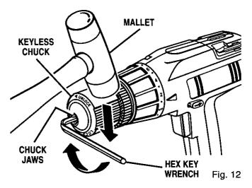
Open chuck jaws and remove hex key wrench. Remove the chuck screw by turning it in a clockwise direction. See Figure 13. Note: The screw has left hand threads.
